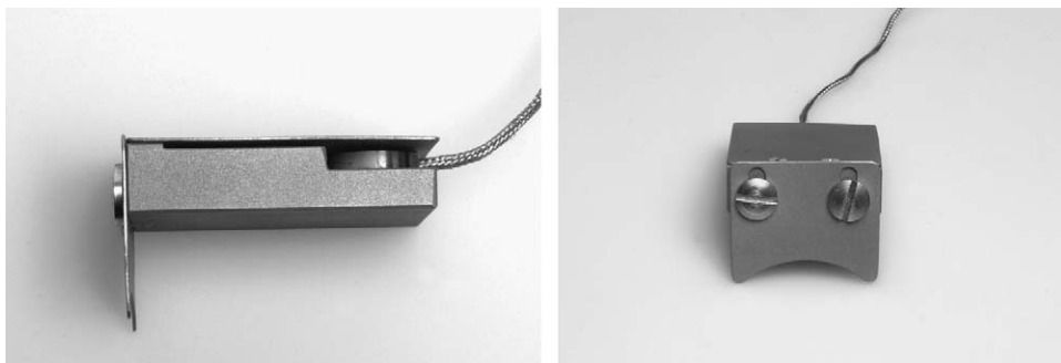
Sensor gauge with integrated force sensor in two projections for measuring the subligamentous forces in the height of the greater trochanter.
