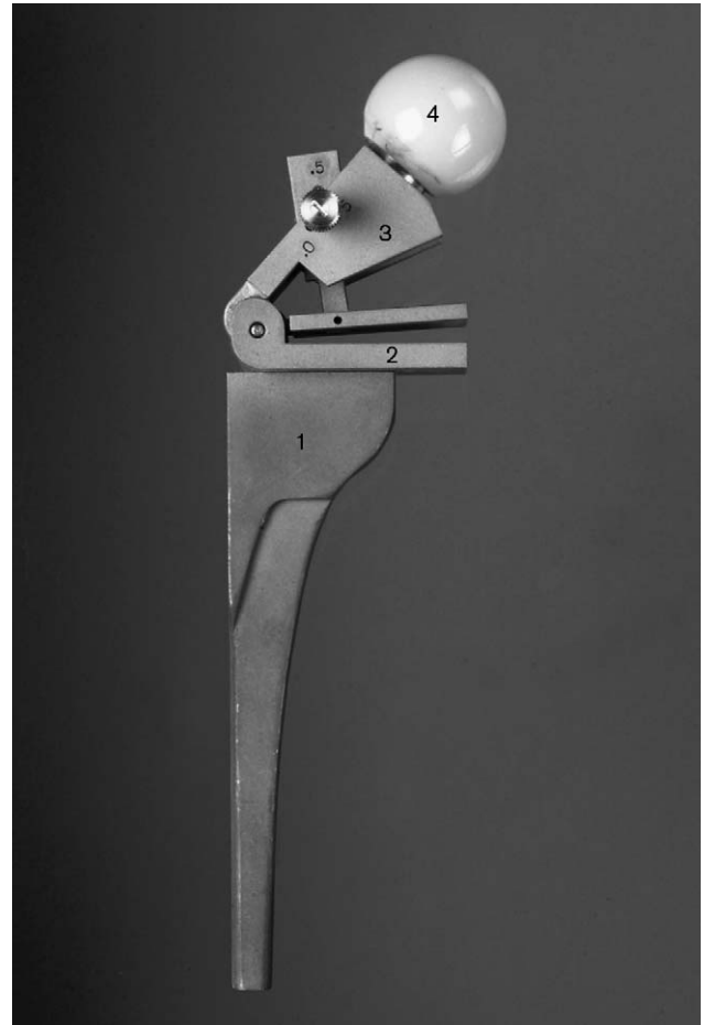
Sensor prosthesis with adjustable collodiaphyseal angles in the height of the femoral neck and with a ceramic head. 1 femoral shaft; 2 ground plate; 3 femoral neck with stick axis; 4 ceramic head; arrow position of the sensor gauge.
